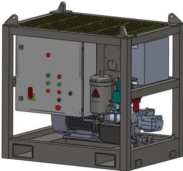
An on-deck or workshop hpu unit for supplying hydraulic power to an ROV system for testing, pre-dive checks, and setup operations. The unit eliminates the need to operate the vehicle HPU out of the water avoiding overheating issues and unnecessary wear and tare.
